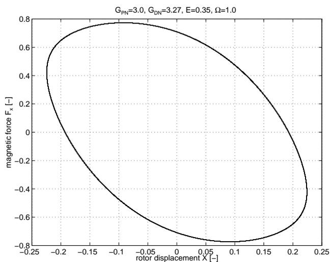
Figure 6. MAGNETIC FORCE IN TERMS OF ROTOR DISPLACEMENT FOR THE PARAMETER SET  $G_{PN} = 3.0$ ,  $G_{DN} = 3.27$ ,  $E = 0.35$  AND  $\Omega = 1.0$ .
