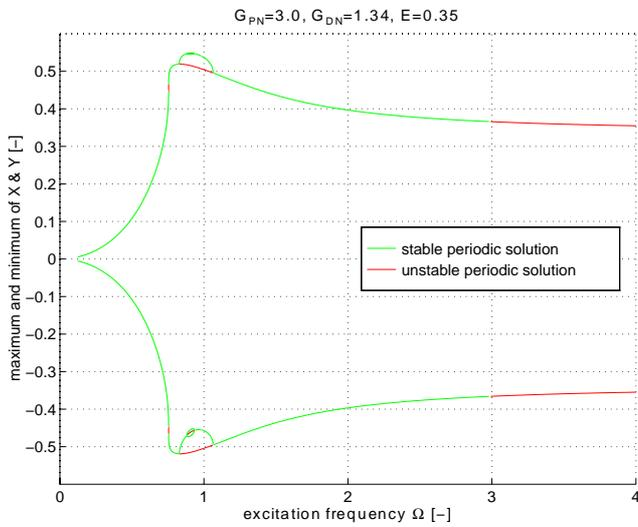
Figure 9. AMB SYSTEM RESPONSE FOR THE PARAMETER VALUES  $G_{PN} = 3.0$ ,  $G_{DN} = 1.34$  AND  $E = 0.35$ . THE PLOT SHOWS MAXIMUM AND MINIMUM OF THE UNSYMMETRIC PERIODIC SOLUTION. MAGNIFICATIONS ARE SHOWN IN FIGURES 10 AND 11.
