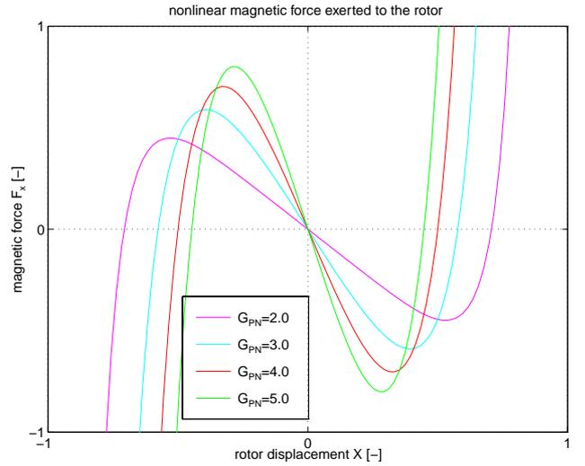
Figure 2. NONLINEAR MAGNETIC FORCE EXERTED TO THE ROTOR WITHOUT DIFFERENTIAL FEEDBACK. THE PROPORTIONAL FEEDBACK  $G_{PN}$  IS VARIED FROM 2.0 TO 5.0.
