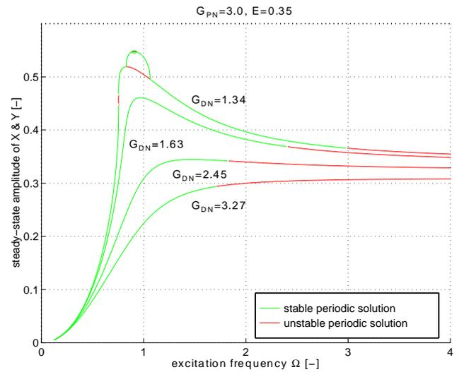
Figure 3. AMB SYSTEM RESPONSE FOR THE PARAMETER VALUES  $G_{PN} = 3.0$  AND  $E = 0.35$ .  $G_{DN}$  IS VARIED FROM 3.27 TO 1.34.
