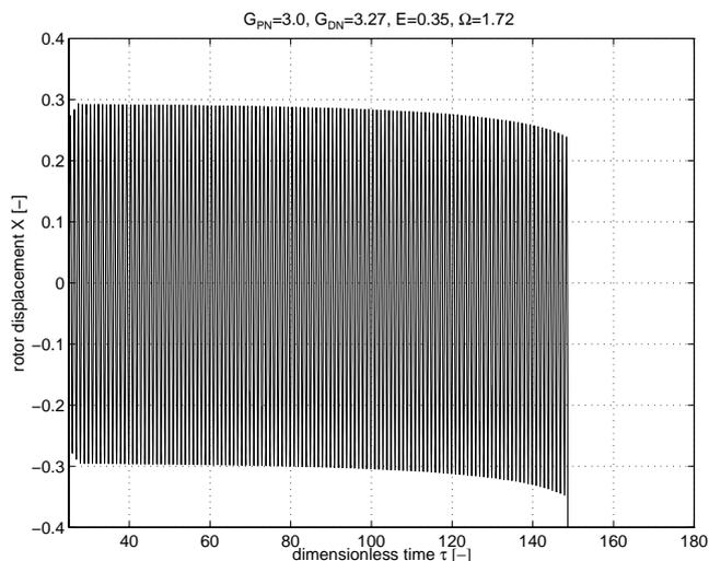
Figure 5. ROTOR VIBRATION IN TERMS OF DIMENSIONLESS TIME  $\tau$  FOR THE PARAMETER SET  $G_{PN} = 3.0$ ,  $G_{DN} = 3.27$ ,  $E = 0.35$  AND  $\Omega = 1.72$ .
