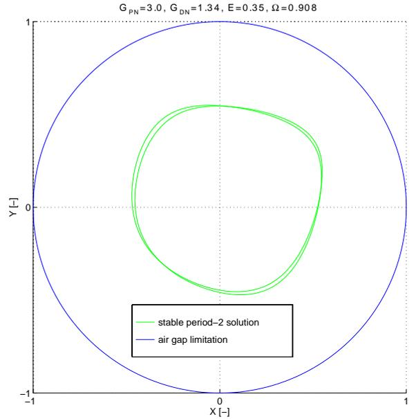
Figure 14. STABLE UNSYMMETRIC SOLUTION WITH PERIOD 2 FOR THE PARAMETER SET  $G_{PN} = 3.0$ ,  $G_{DN} = 1.34$ ,  $E = 0.35$  AND  $\Omega = 0.908$ .
