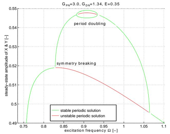
Figure 10. AMB SYSTEM RESPONSE FOR THE PARAMETER VALUES  $G_{PN} = 3.0$ ,  $G_{DN} = 1.34$  AND  $E = 0.35$ . DETAIL OF FIGURE 9.
