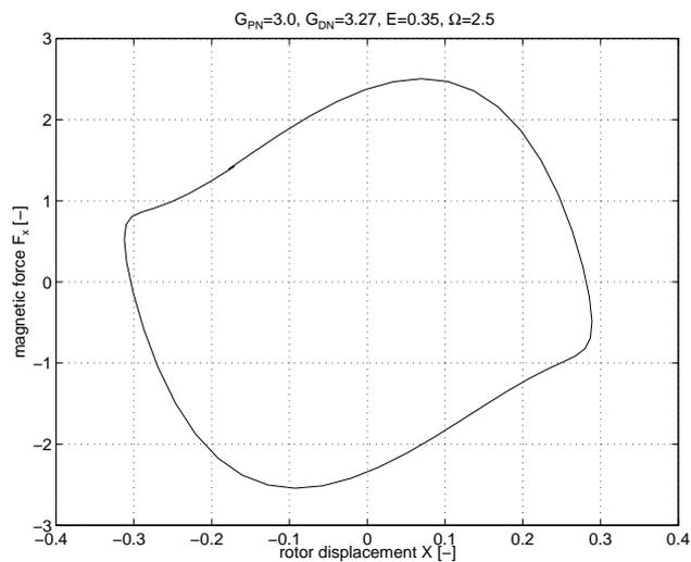
Figure 8. MAGNETIC FORCE IN TERMS OF ROTOR DISPLACEMENT FOR THE PARAMETER SET  $G_{PN} = 3.0$ ,  $G_{DN} = 3.27$ ,  $E = 0.35$  AND  $\Omega = 2.5$ .
