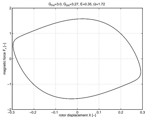
Figure 7. MAGNETIC FORCE IN TERMS OF ROTOR DISPLACEMENT FOR THE PARAMETER SET  $G_{PN} = 3.0$ ,  $G_{DN} = 3.27$ ,  $E = 0.35$  AND  $\Omega = 1.72$ .
