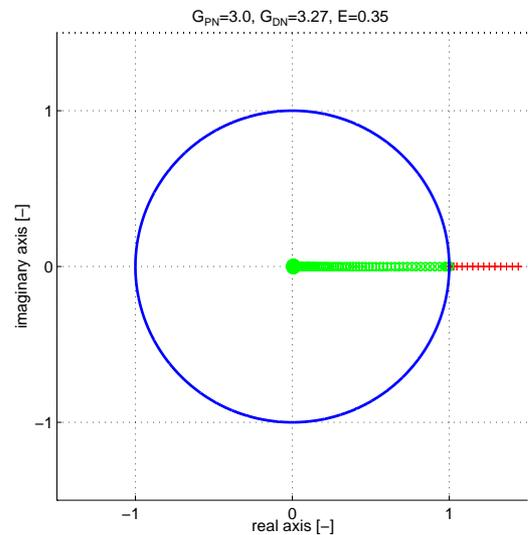
Figure 4. EIGENVALUES OF THE MONODROMY MATRIX FOR THE PARAMETER SET  $G_{PN} = 3.0$ ,  $G_{DN} = 3.27$  AND  $E = 0.35$ .  $\Omega$  IS VARIED FROM 0.1 TO 1.87.
