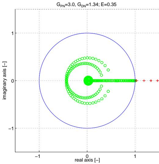
Figure 12. EIGENVALUES OF THE MONODROMY MATRIX FOR THE PARAMETER SET  $G_{PN} = 3.0$ ,  $G_{DN} = 1.34$  AND  $E = 0.35$ .  $\Omega$  IS VARIED FROM 0.1 TO 0.85.
