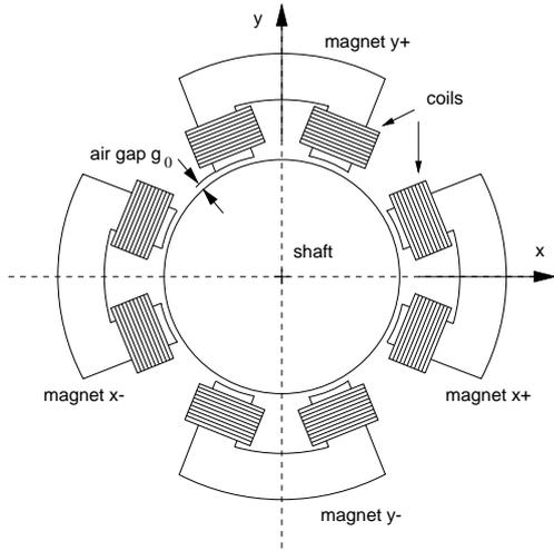
Figure 1. SCHEMATIC OF AN ACTIVE MAGNETIC BEARING WITH SHAFT IN CENTER POSITION.
