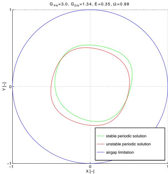
Figure 13. STABLE UNSYMMETRIC SOLUTION AND UNSTABLE SYMMETRIC SOLUTION FOR THE PARAMETER SET  $G_{PN} = 3.0$ ,  $G_{DN} = 1.34$ ,  $E = 0.35$  AND  $\Omega = 0.98$ .
