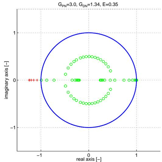
Figure 15. EIGENVALUES OF THE MONODROMY MATRIX FOR THE PARAMETER SET  $G_{PN} = 3.0$ ,  $G_{DN} = 1.34$  AND  $E = 0.35$ .  $\Omega$  IS VARIED FROM 0.83 TO 0.9.
